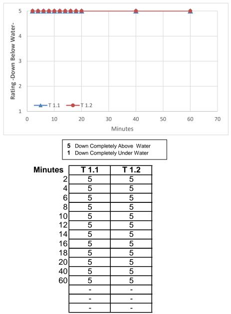
Treated material remains at a rating of 5 after an average of: 60 minutes
