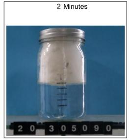
Rating: 5 IDFB 18-A Hydrophobic Shake Test Measured Time Interval – 2 Minutes
