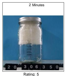
**IDFB 18-A** Hydrophobic Shake Test Measured Time Interval – 2 Minutes
